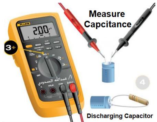
Capacitor measuring and
