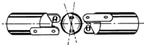
Fig. 2 A pinned sphere shaft coupling replaces a cross-piece. The result is a more compact joint.
