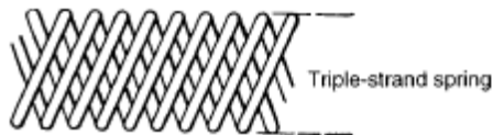
Fig. 8 This flexible shaft permits any shaft angle. These shafts, if long, should be supported to prevent backlash and coiling.
