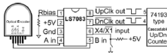
Figure 5.32: An optical encoder, US Digital LS7083
