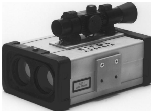
Figure 5.71: The class 1 (eye-safe) LD90-3 series TOF laser rangefinder is a self-contained unit available in several versions with maximum ranges of 150-1500 m under average atmospheric conditions.
