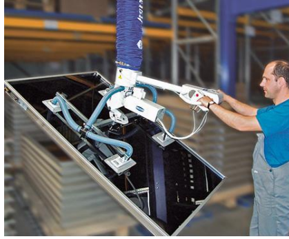
Figure 3.67: Vacuum lifters, vacuum lifts & lifting devices
