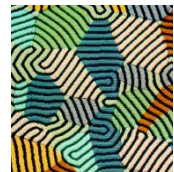
Magnetic domains garnet film 11 \mu m wide stripes
